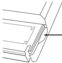
Replace with 2 AA Alkaline Batteries. High quality Alkaline batteries are recommended.
