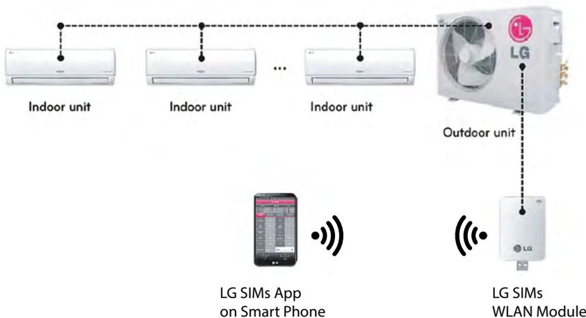
Figure 102: SIMS WLAN Module to Typical DFS System
