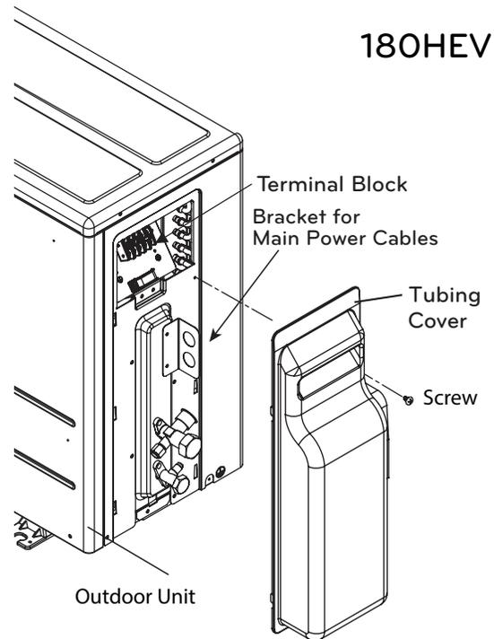
Figure 54: Outdoor Unit Piping Connection (180HEV)
