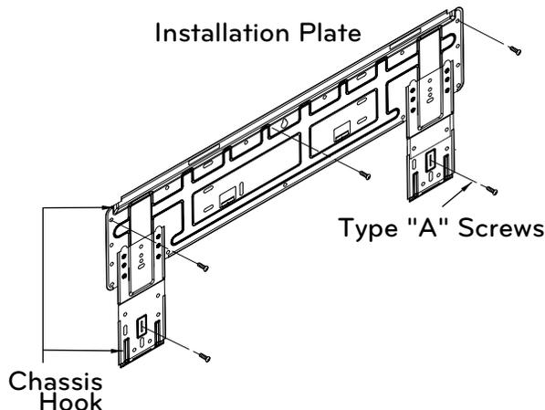
Refer to "Drilling Piping Hole in the Wall" on page 28 as you follow procedure to install plate.
