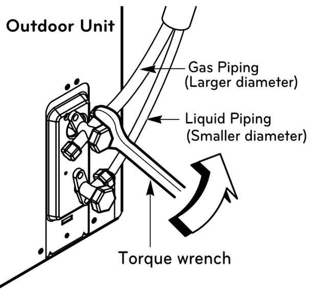
Table 27: Torque Wrench Tightening
