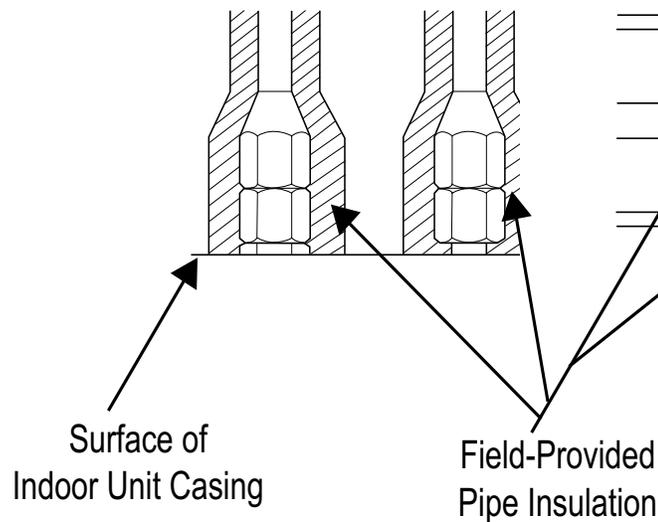
Figure 71: Typical Refrigerant Flare Fitting Insulation Detail
