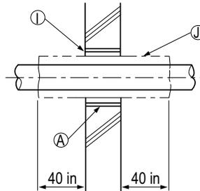
When filling an access hole with mortar, cover the area with steel plate so that the insulation will not fall through. For this area, use fire-resistant materials for both the insulation and cover. (Vinyl cover should not be used.)
