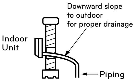
Figure 45: Correct Slope Angle for Drain Hose
