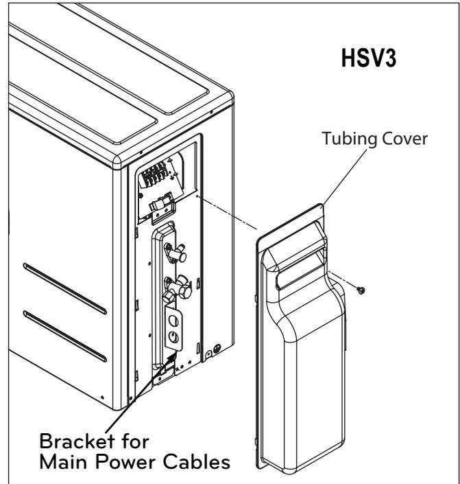
Figure 47: Outdoor Unit Connection Cover Removal (HV3, HLV)
