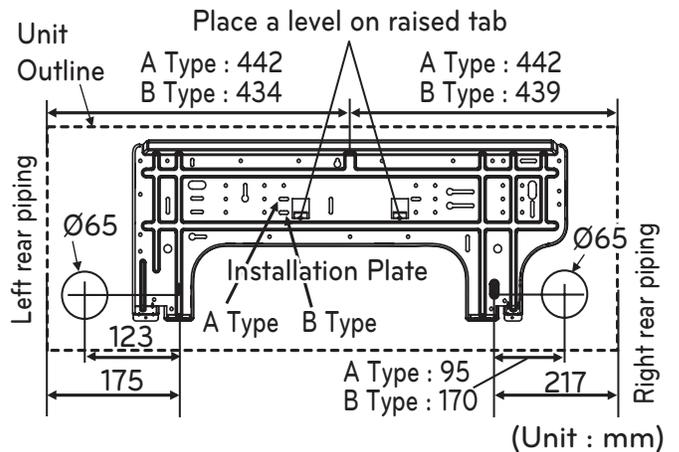
Figure 7: Installation Plate Screws
