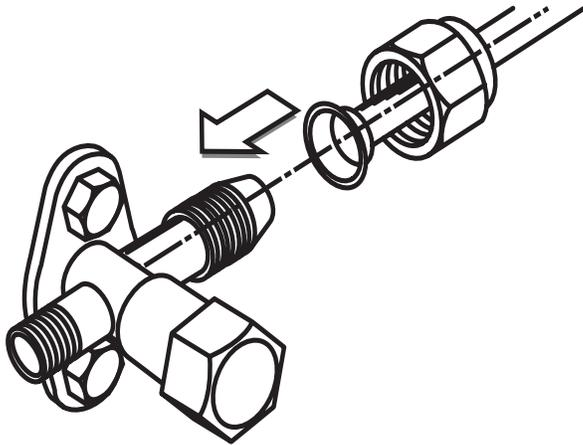
Figure 49: Outdoor Unit Piping Connection (HSV3)
