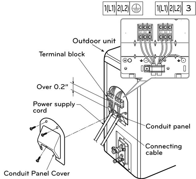
Figure 96: 090HXV, 120HXV Outdoor Unit - Electrical Connections
