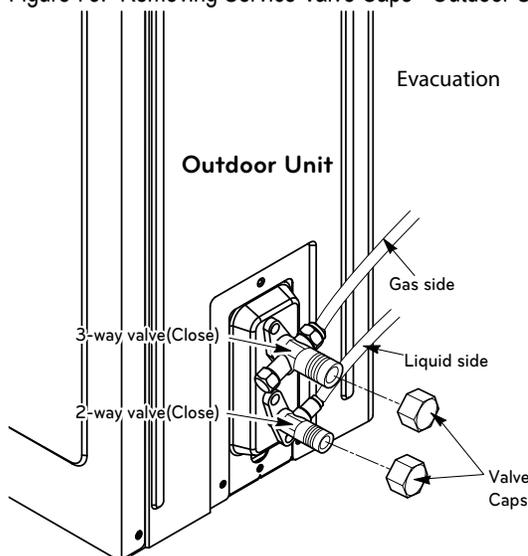
Figure 74: Evacuation Setup
