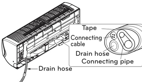
Figure 64: Piping with Insulation Material
