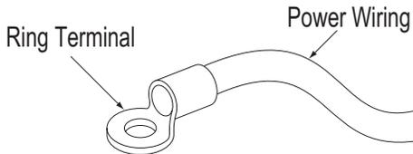
Figure 79: Proper and Improper Power Wiring Connections
