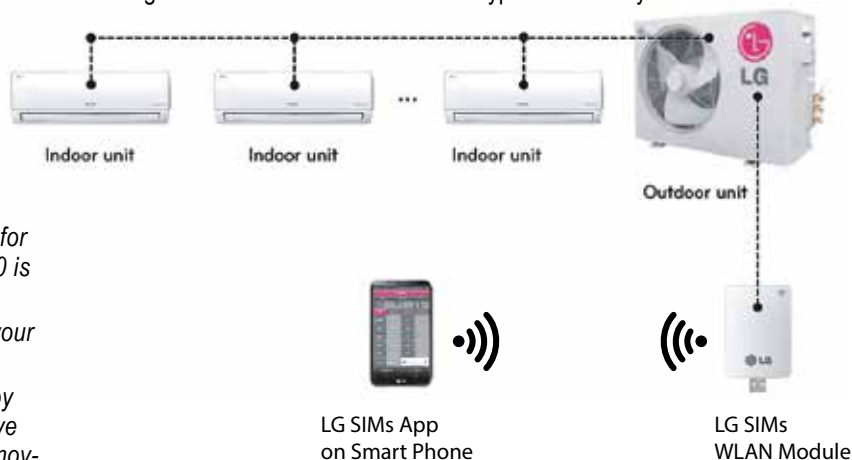
Figure 64: SIMS WLAN Module to a Typical Multi F System.
