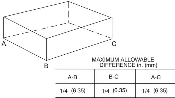
**Fig. 6 - Unit Leveling Tolerances**
